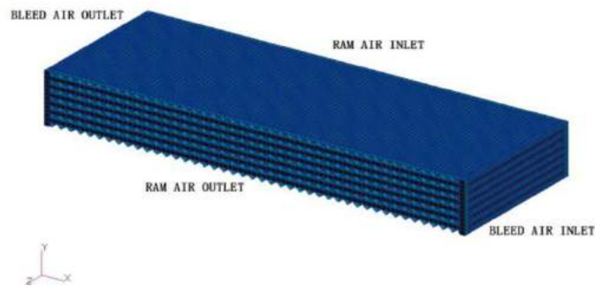
Figure 5.18 Finite element model of radiator core fluid media
