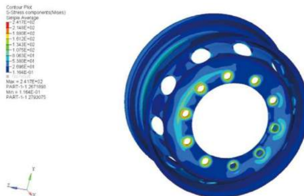
Figure 6-10 Stress nephogram of wheel under bending load
