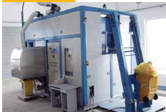
MICROWAVE DISINFECTION TREATMENT FACILITY FOR MEDICAL WASTE
